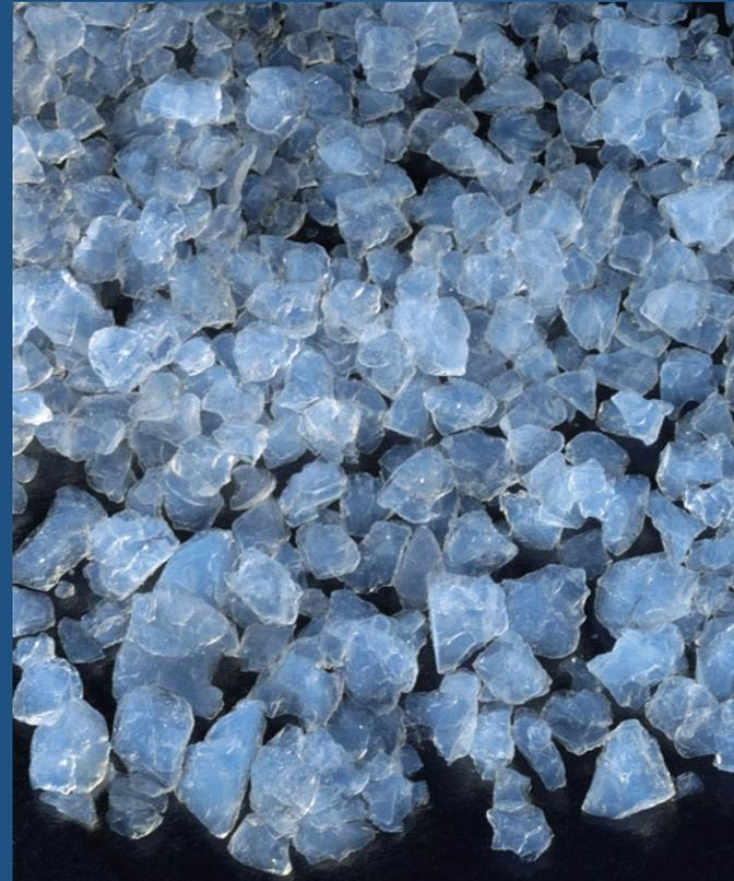
*Silica aerogel insulation granules
