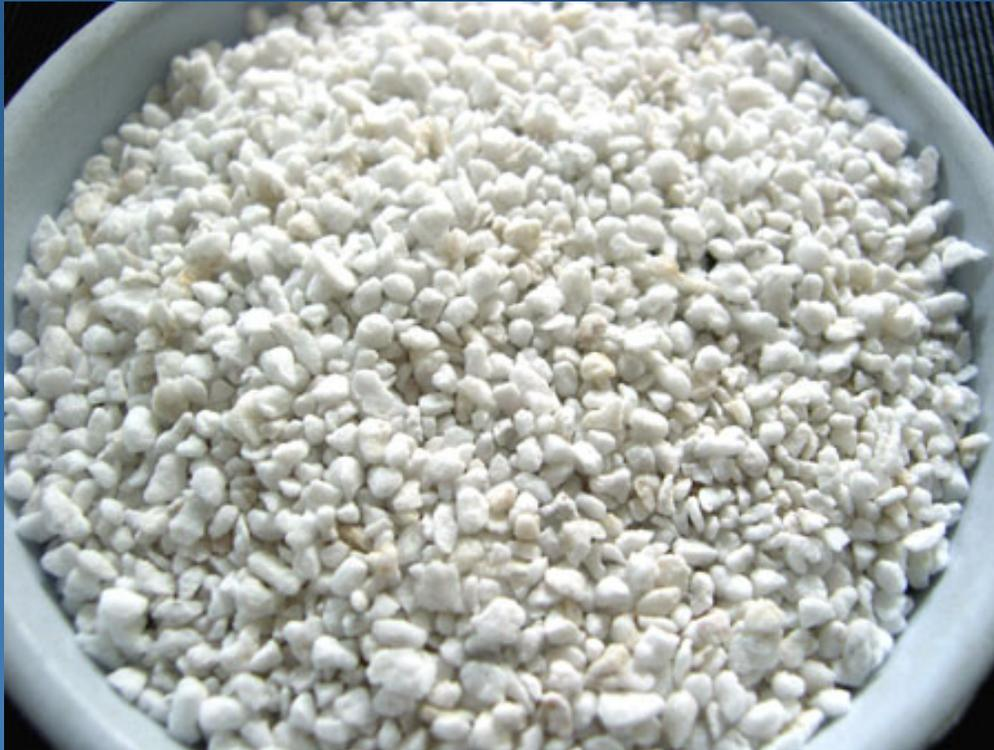
*Perlite insulation – photo: DFL Minmet Refractories Corp*
