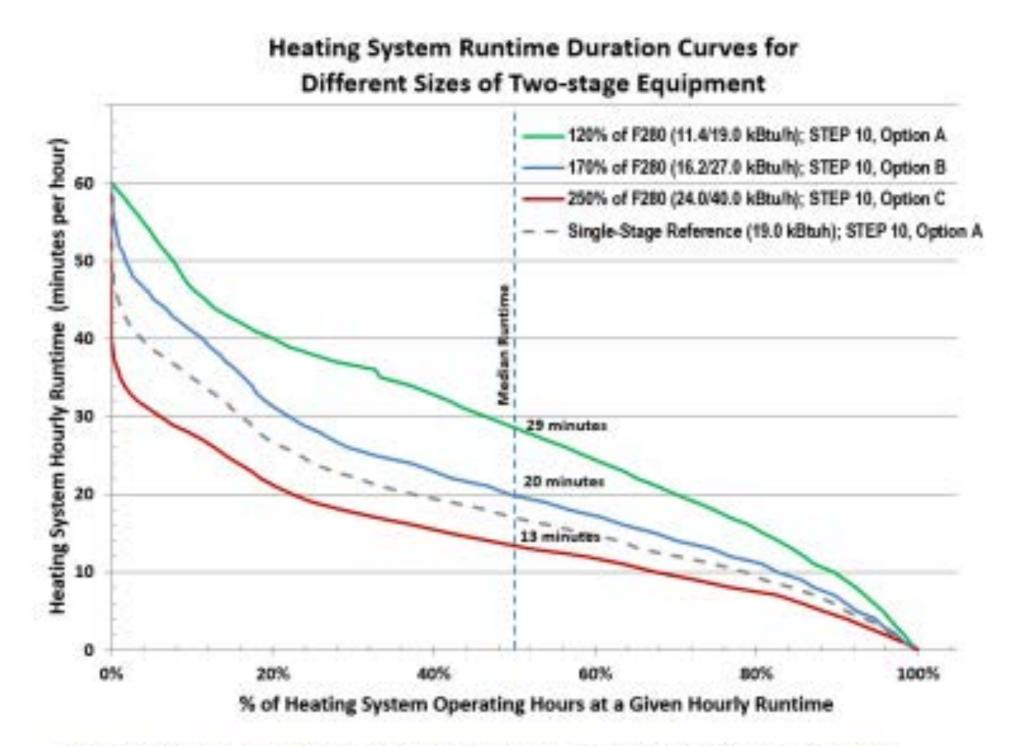
Figure 22: Runtime Duration Curves for Two-Stage Equipment
