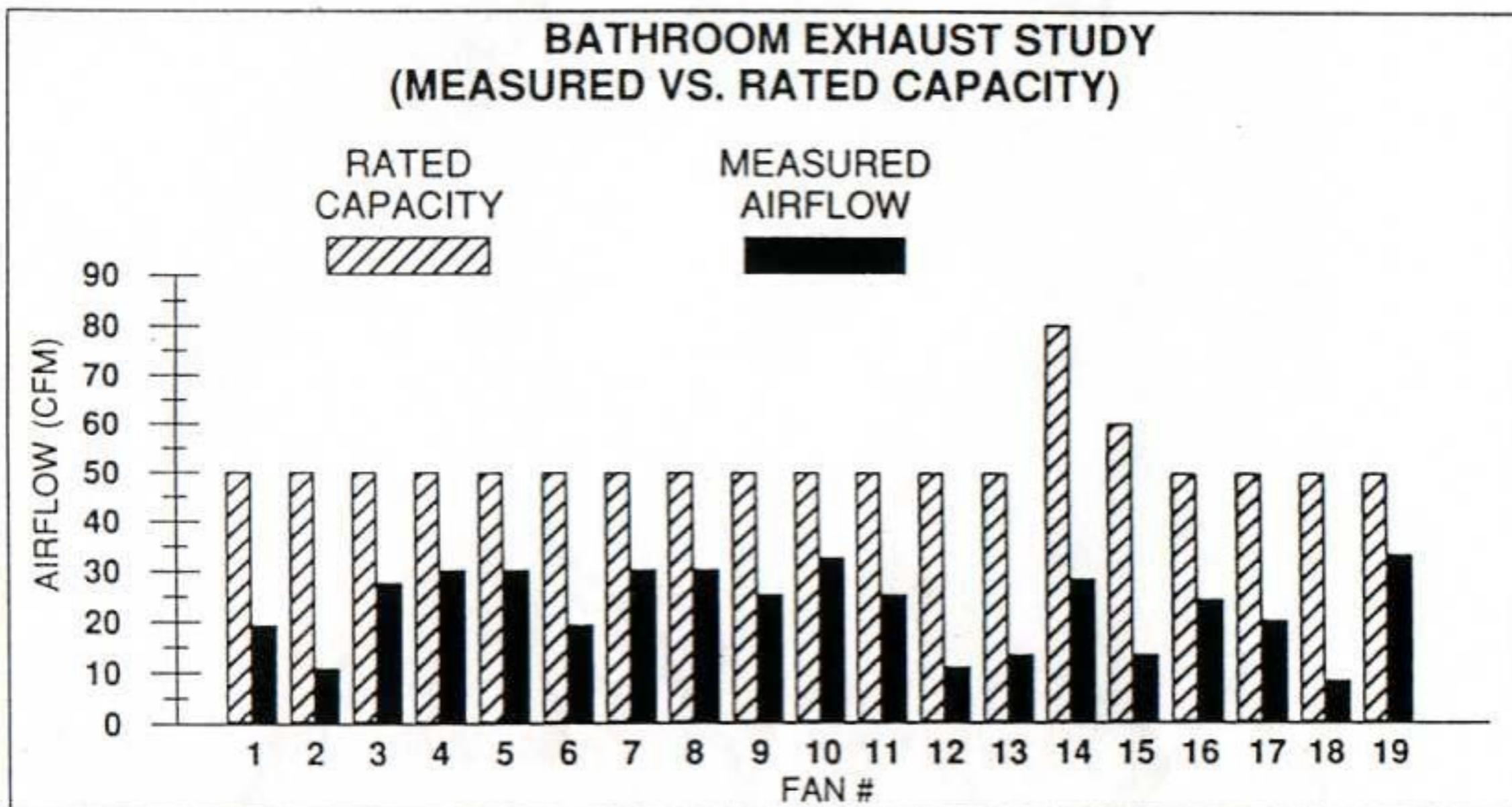
Canadian bathroom exhaust study. In 26 fans tested (19 shown here), the measured airflow of the installed fan was less than half the rated capacity in nearly every case.
