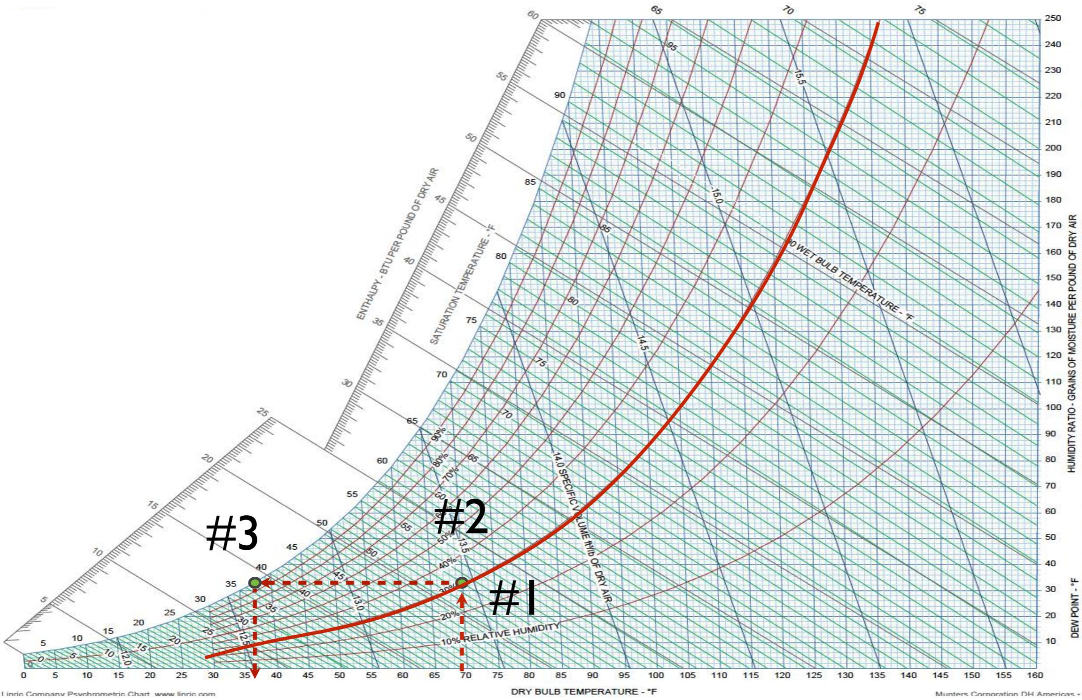
a) If indoor air is at 70 F and 50% RH, to what temperature must it be cooled to get condensation? **50.53 F** This is the Dew Point
