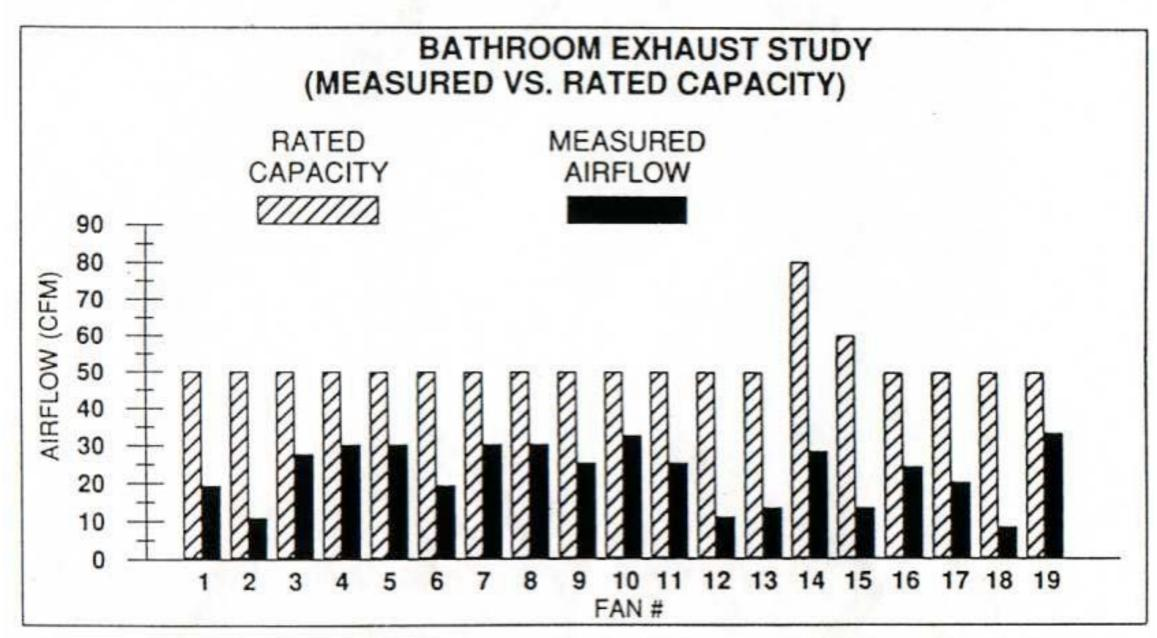
Canadian bathroom exhaust study. In 26 fans tested (19 shown here), the measured airflow of the installed fan was less than half the rated capacity in nearly every case.
