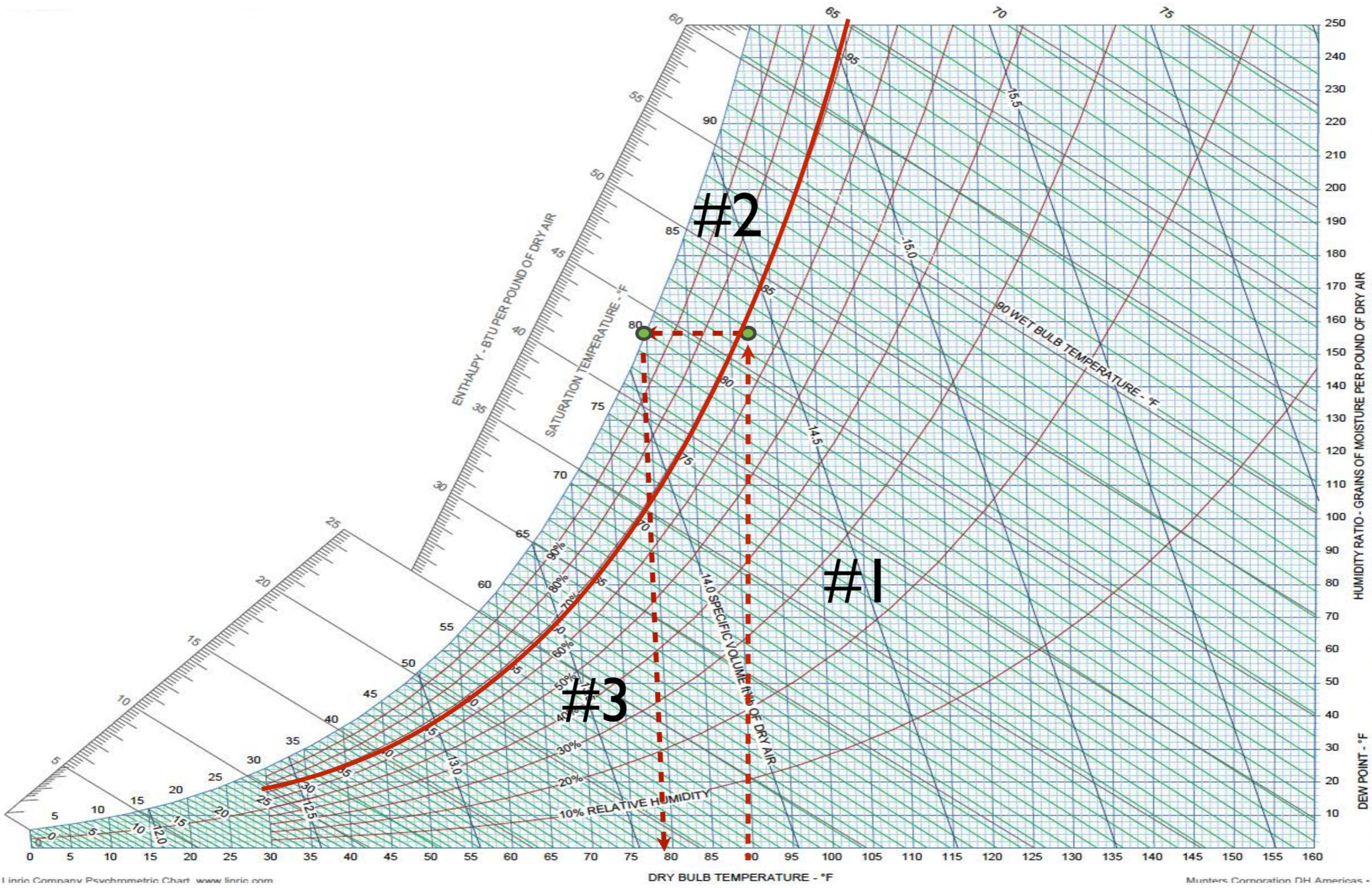
2. If the outside air is 25 F and 100% RH, what will the RH be of the air once it is brought in and warmed up to 70 F? **19.0 %**
