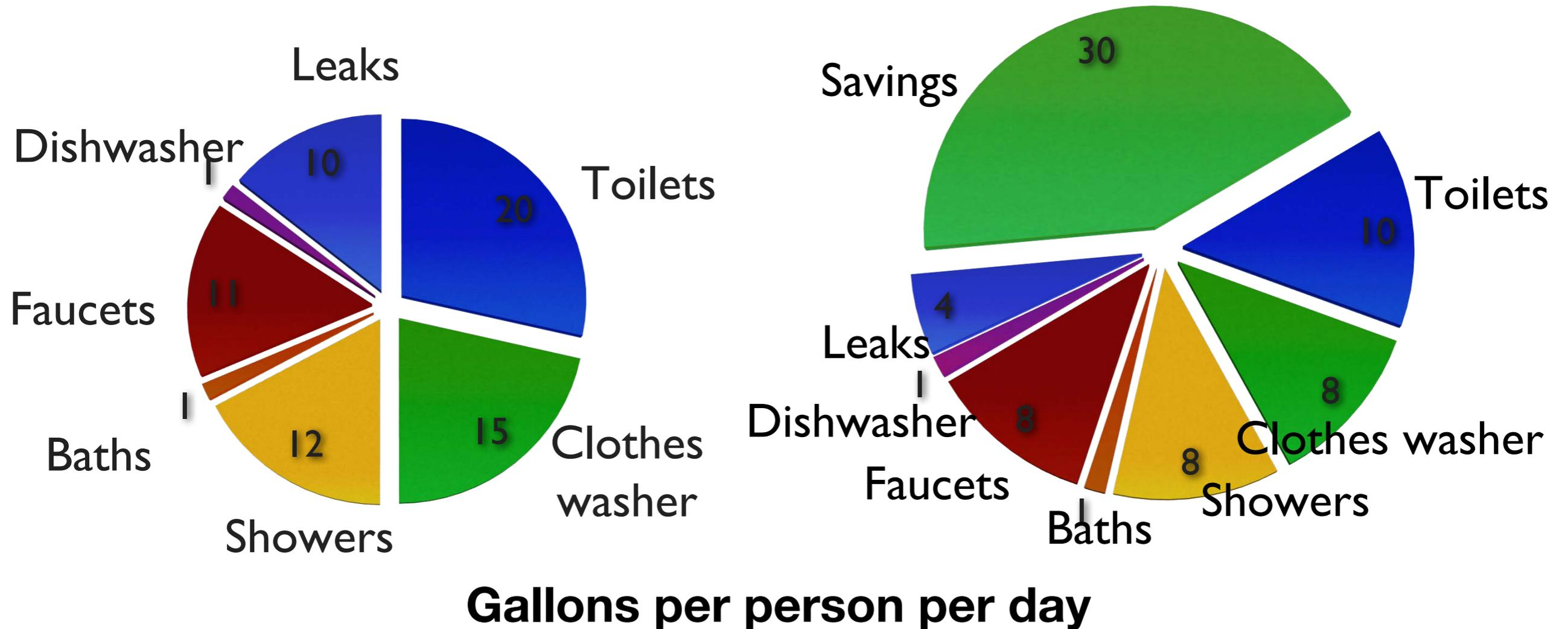
An EPA water efficiency retrofit study indicated the total water use was reduced to 40 gallons per person per day - 39% reduction
