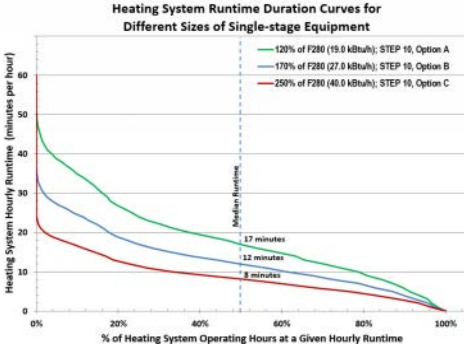
Figure 21: Runtime Duration Curves for Single-Stage Equipment
