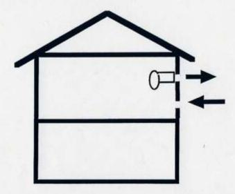
Makeup air is intended to limit the negative pressure in the home when exhaust devices are in operation.
