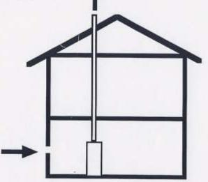
Combustion air is intended to ensure proper combustion and venting of combustion by-products.
