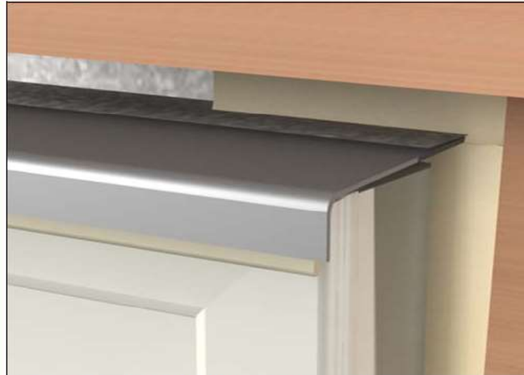
Figure 22 Apply sealant between window and exterior finish.
