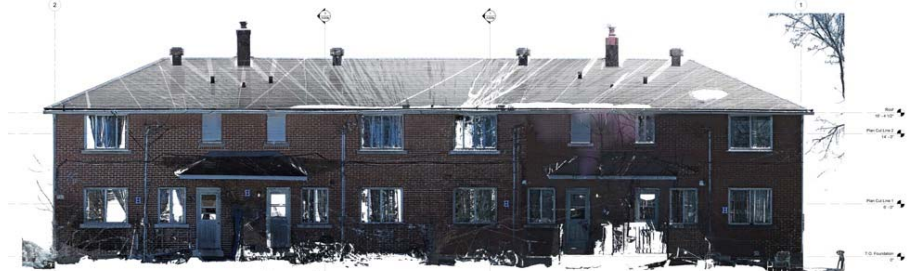
2 North Elevation (Point Cloud) 3/8" = 1'-0"
