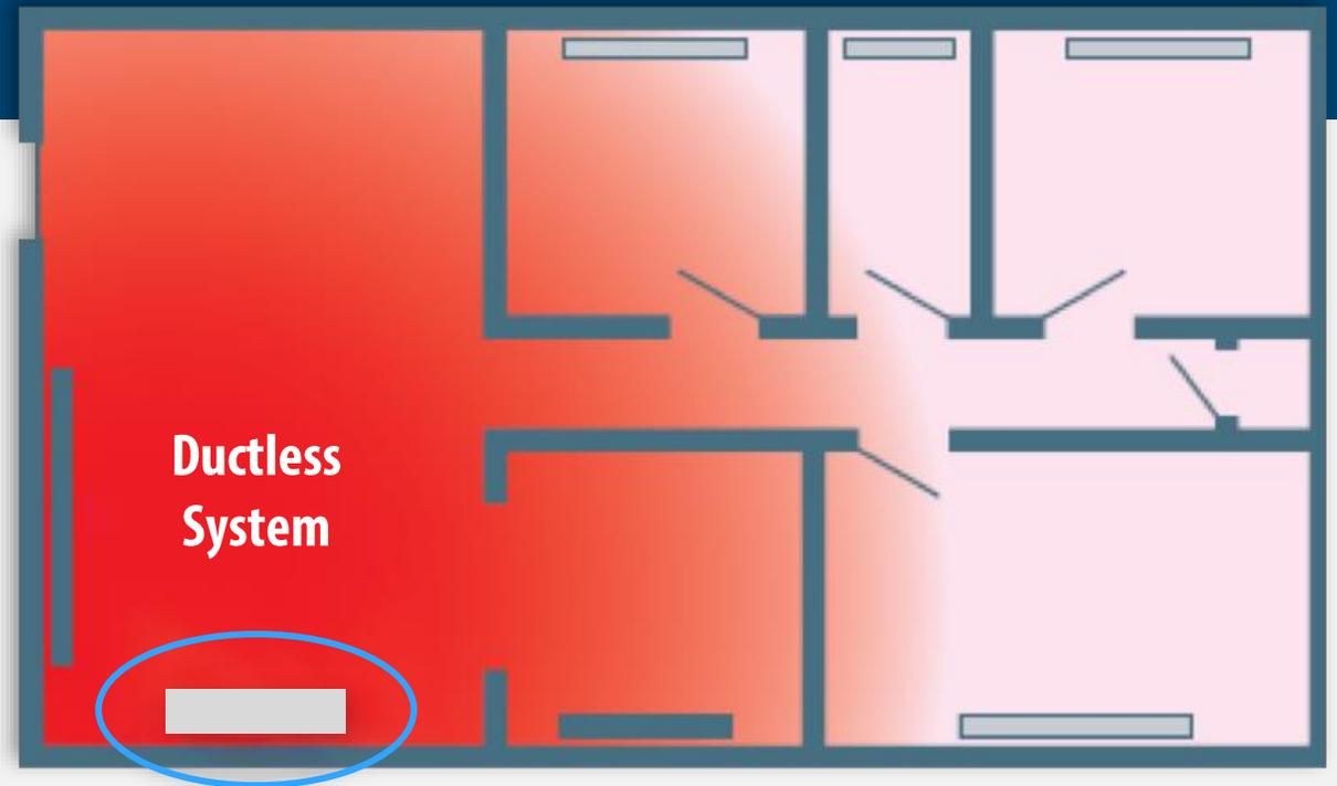
**DISPLACEMENT SOLUTION:** Single-head ductless system in primary living area; existing heat remain used as back-up.
