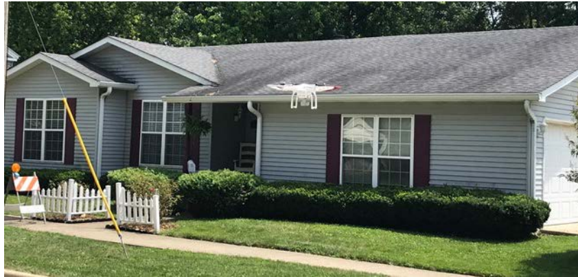
360-degree building scan performed in <15 minutes with a spatial accuracy of <1 mm
