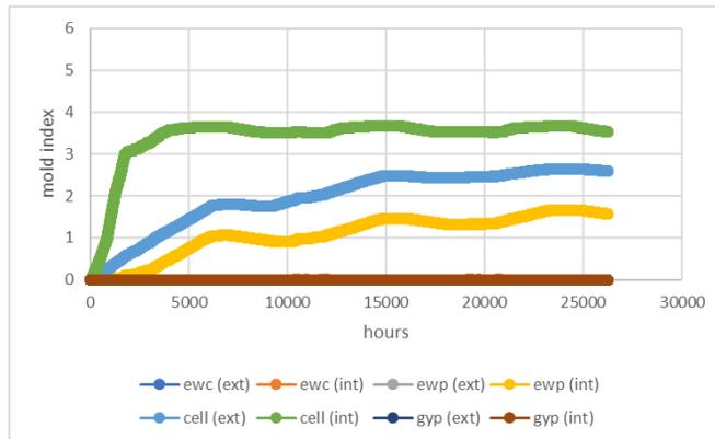
Note: The hygrothermal properties are used to calculate a mold index based on the VTT model for all surfaces, excluding WRBs, and then classified in accordance with ASHRAE 160. Mold index is used to compare different wall retrofits.
