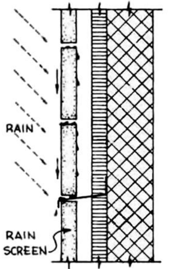
WATER THAT PENETRATES IS DIVERTED OUTWARD BY FLASHINGS
