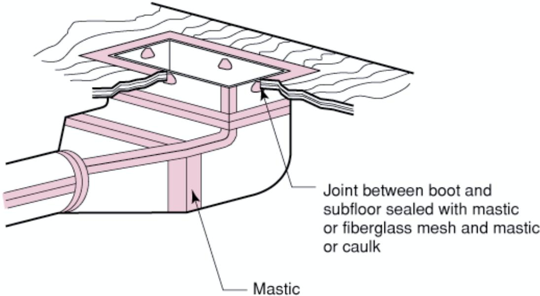
Joint between boot and subfloor sealed with mastic or fiberglass mesh and mastic or caulk
