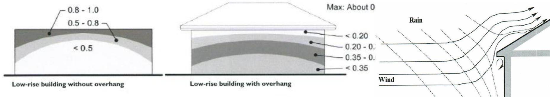
Figure A3-3 Typical rain wetting pattern on low-rise buildings (Straube and Burnett 2005).
