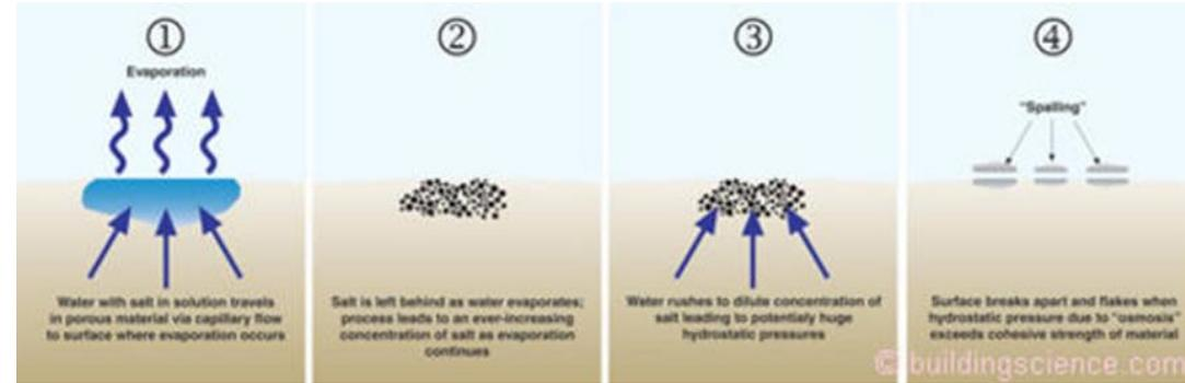
Spalling of porous materials—Without salt present evaporation of water from porous surfaces can often be easily managed—with salt present significant damage can occur.
