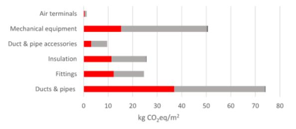
Figure 4. Climate change impact results for the assessed HVAC categories in kgCO2eq/m<sup>2</sup>.
