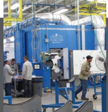
From left: Dropping the ceiling height in the paint preparation area has reduced the number of dust collectors needed to control indoor air quality, while lowering HVAC costs. This design improvement is being replicated in the new building. Bright, white, energy-efficient LED lights help ensure perfection in every plane. Cirrus Aircraft is ramping up production on the FAA certified Vision Jet.
