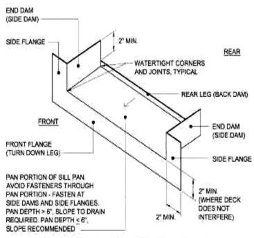
FIG. A3.4 Configurations of Typical Still Pan Flashing-Isometric
