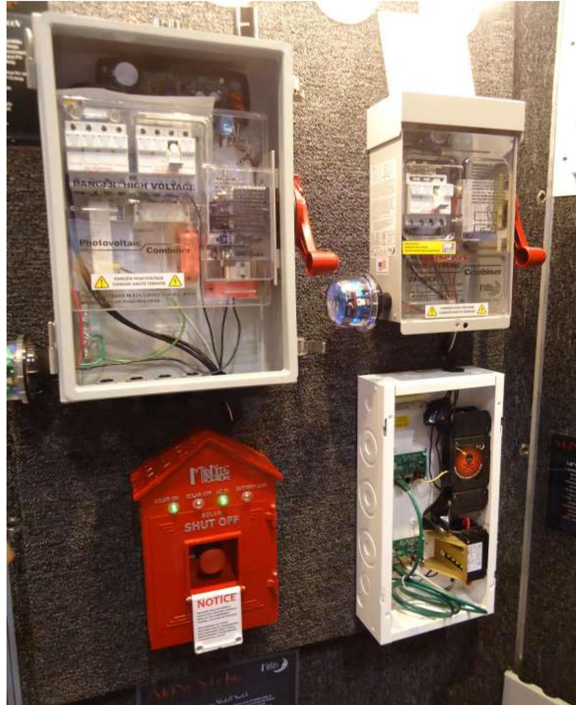
Combiner Boxes now offer integral disconnecting means... MidNite Solar's offers a hard wired remote called the "Birdhouse" to be located at the service entrance... while this is the one solution that can work with battery based systems to rapidly shut down the entire DC system it does not comply with the 2019 requirements for Module level RDS.
