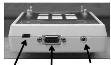
USB Serial Fan Control Communication Communication Output Jack Port Port
