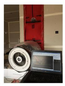
Blower door setup for pressurization
