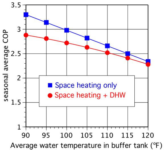
With full outdoor reset of tank temperature + **all electric resistance heat for DHW**
