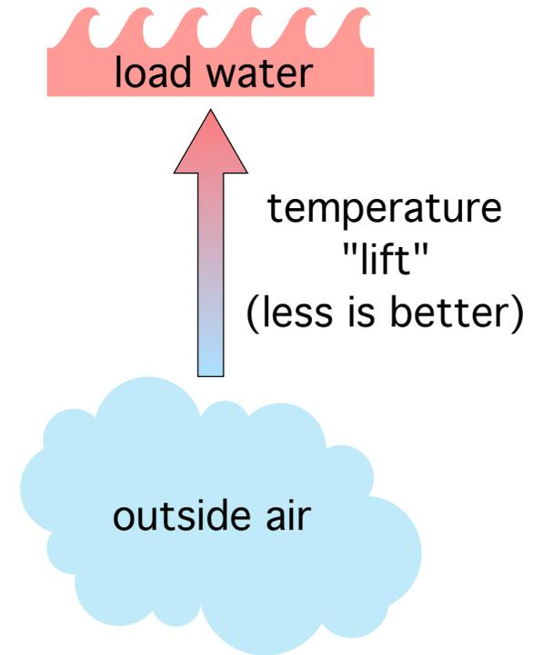
**Anything that *reduces* the “temperature lift” *increases* both the heating capacity and COP of the heat pump.**
