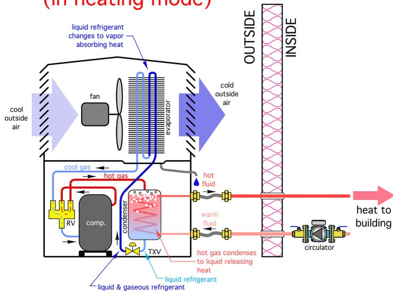
In heating mode: The heat pump extracts low temperature heat from outside air, and transfers it to a fluid stream (water or water & antifreeze) to be used by a hydronic distribution system.
