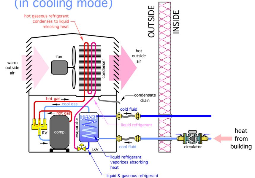
In cooling mode: The heat pump extracts low temperature heat from a fluid stream (chilling it), and dissipates that heat to outside air.
