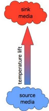
The smaller the "temperature lift" between evaporator and condenser, the higher the heating capacity and COP.
