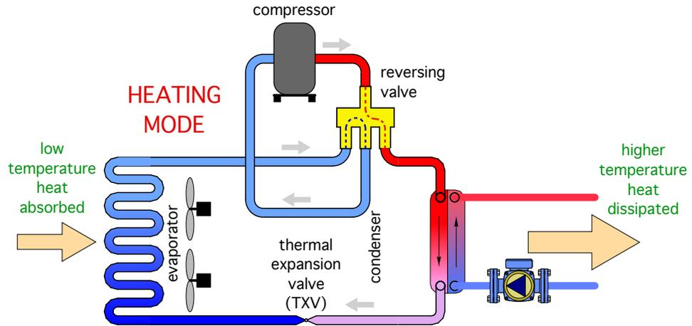
A brazed-plate stainless steel heat exchanger is the refrigerant-to-water heat exchanger (e.g., **condenser**) during **heating** mode.
