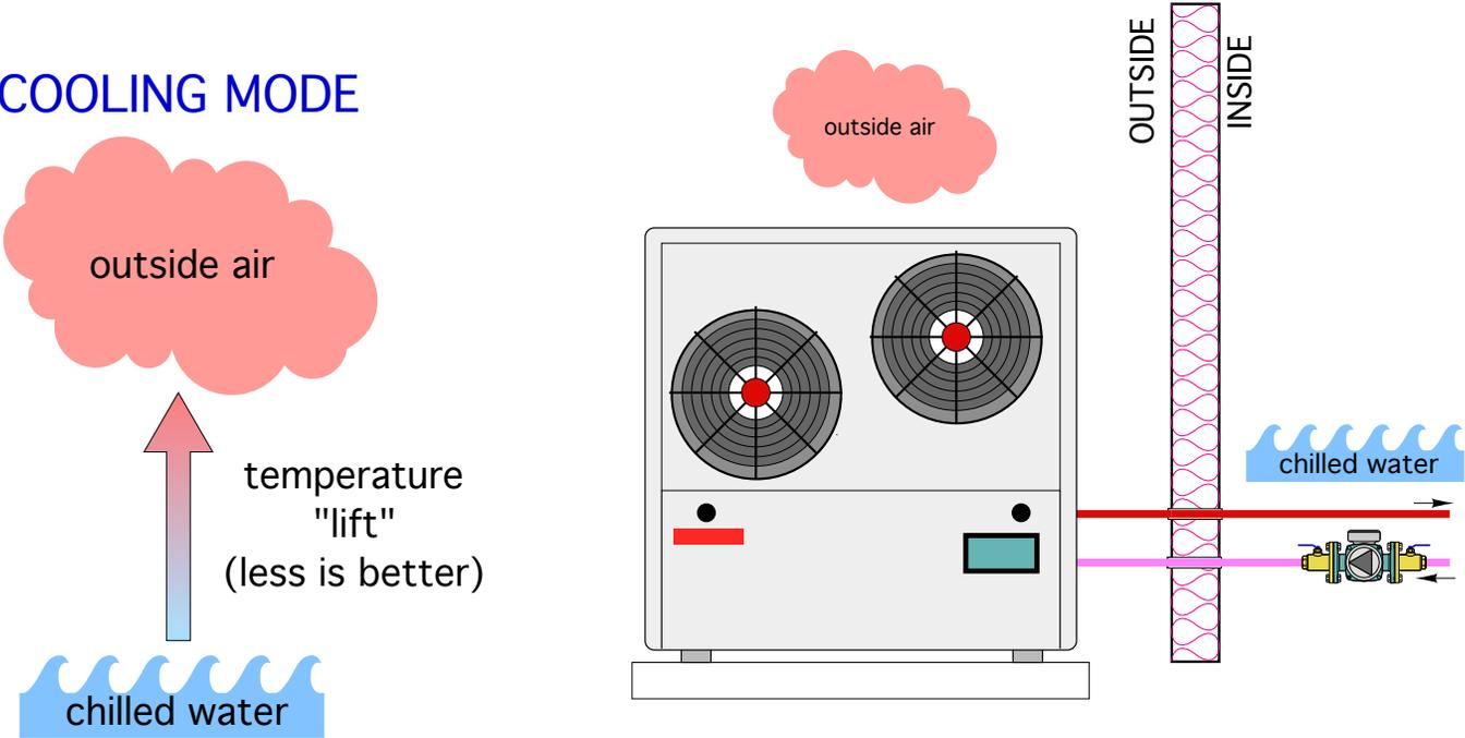
**Anything that decreases the temperature lift' increases both the cooling capacity and EER of the heat pump.**
