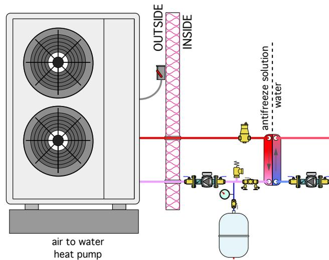
Use 25-40% propylene glycol in the heat pump loop, with water in remainder of system.
