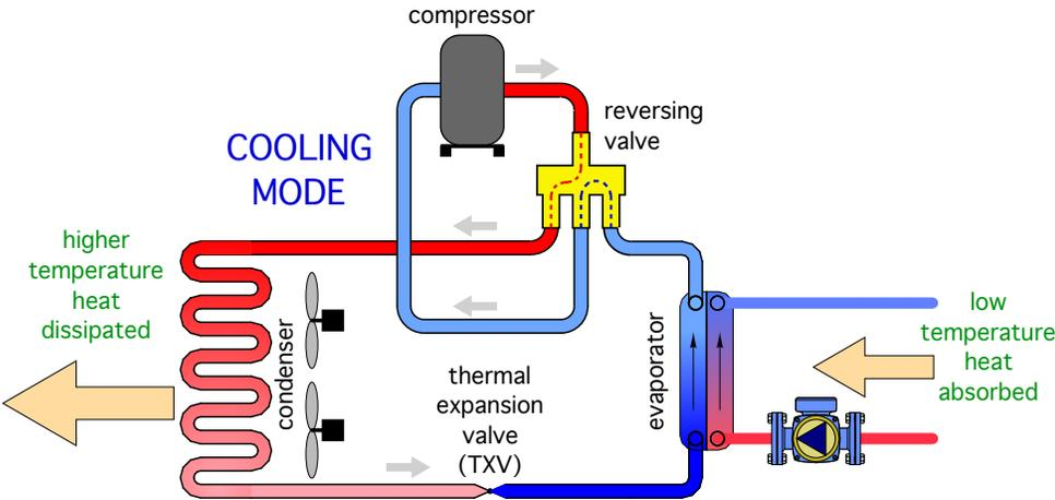
A brazed-plate stainless steel heat exchanger is the refrigerant-to-water heat exchanger (e.g., **evaporator**) during **cooling** mode.
