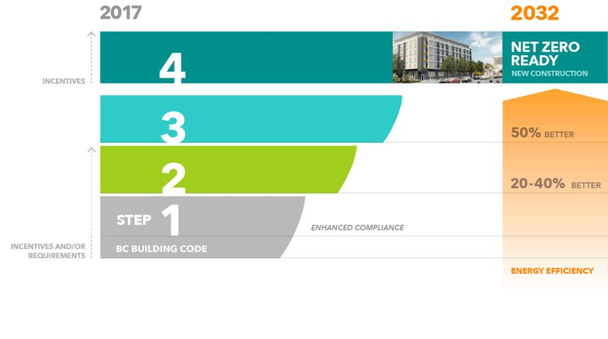
To comply with the BC Energy Step Code, builders must use **energy software modeling** and **on-site testing** to demonstrate that both their design and the constructed building meet the requirements of the standard. They may use any materials or construction methods to do so.
