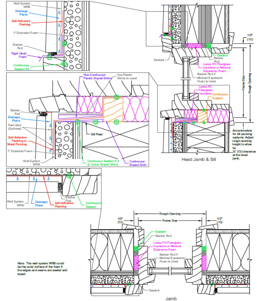
Note: The wall system WRB could be the outer surface of the foam if the edges and seams are sealed and taped.
