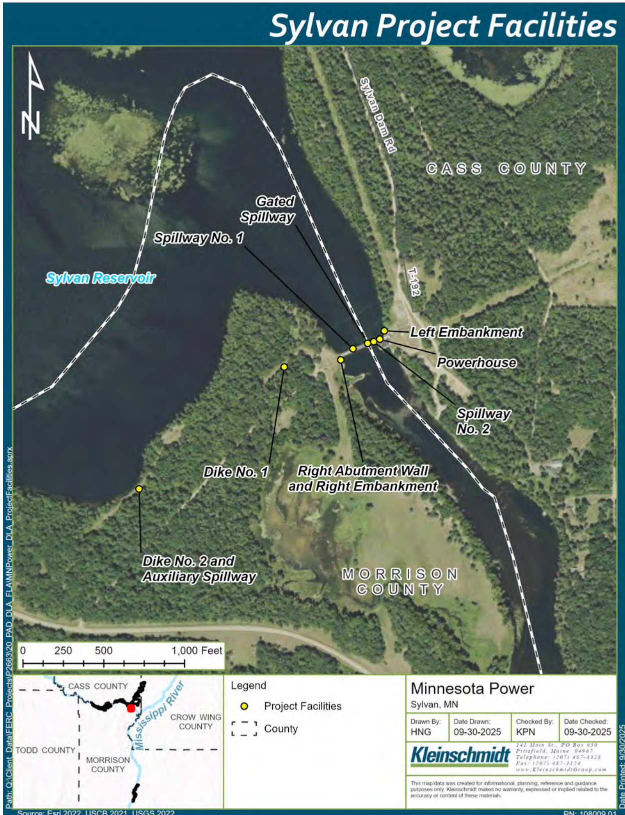
Figure 3-2: Sylvan Project Facilities
